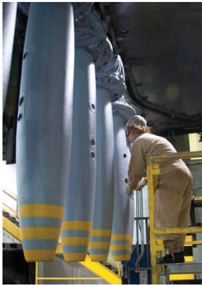
McAlester Army Ammunition Plant employee checks the correct filling of a general purpose bomb.
