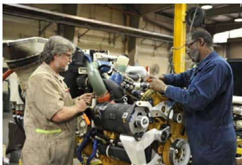
An Anniston Army Depot mechanic and a General Dynamics Land Systems mechanic work on a Stryker power pack.
