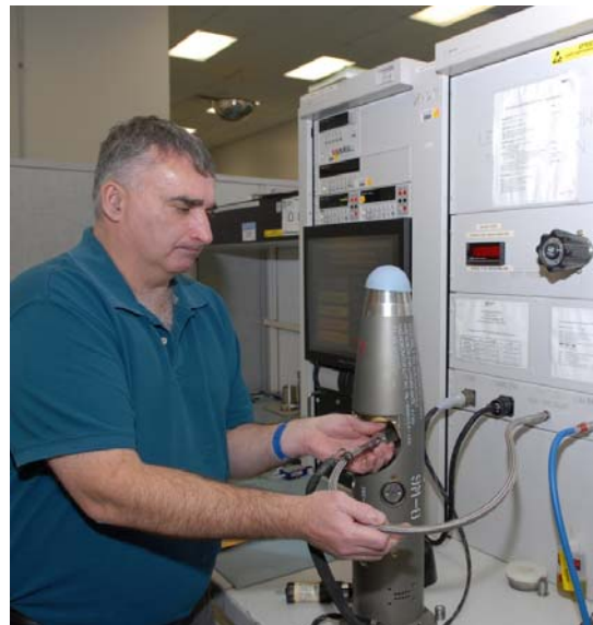
An electronics mechanic at Tobyhanna (Pennsylvania) Army Depot, performs a leak and flow test on a Sidewinder missile guidance and control section.
