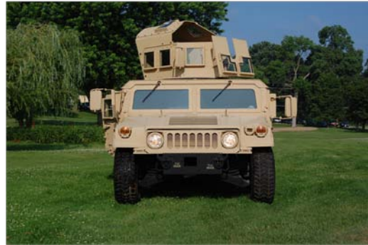
Up-armored HMMWV equipped with Objective Gunner Protection and Overhead Protection cover manufactured at Rock Island Arsenal.
